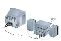
To connect to a hi-fi system, use an audio onnection cable and connect the "L" and "R" outputs on the TV set to the "AUDIO IN" "L" and "R" input on your hi-fi amplifier. Make the connections as shown.
